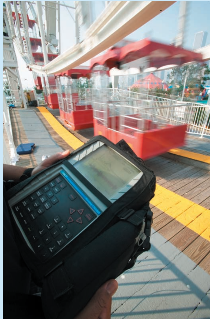
An SKF Microlog® portable data collector, which collects vibration data from sensors attached to the Ferris Wheel's bearings.
