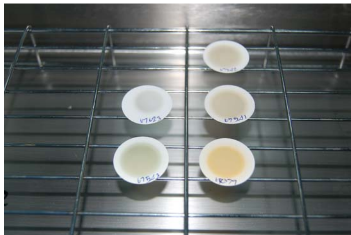
Figure 1. VPI Patches with Stains in Drying Process
